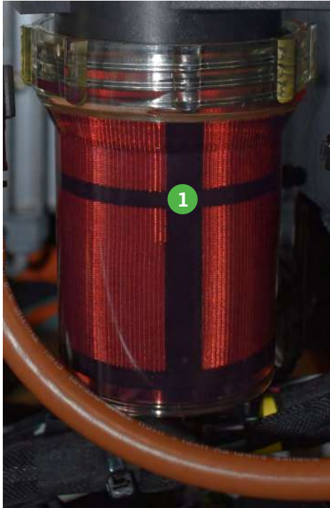
1 NEW: Enhanced Fuel Filtration that supports common-rail fuel injection.
