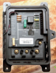
Power Control Module
